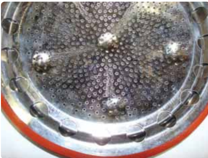
Figure 143 Inspecting interior and cleaning the burner
