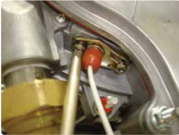
Figure 138 Removal of Ignition electrode
