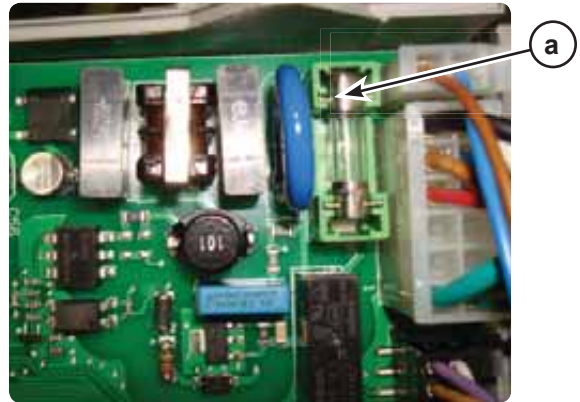
Figure 112 Thermostat-relay circuit fuse location
